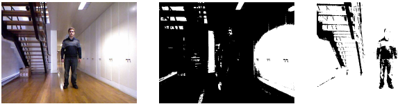
Fig. 5: From left to right, an example of an image acquired in auto mode by the camera the autonomous service robot, the corresponding white areas obtained autonomously, and the corresponding black areas also obtained autonomously by the proposed algorithm.
