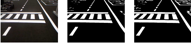
Fig. 4: From left to right, an example of an image acquired in auto mode by the camera the autonomous driving robot, the corresponding white areas obtained autonomously, and the corresponding black areas also obtained autonomously by the proposed algorithm.
