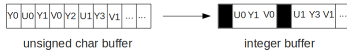
Figure 9: An illustration of the conversion of the unsigned char buffer to an integer one, allowing thus the reading of 4 bytes at the same time. Using this approach we can obtain a reduced resolution of the images.
