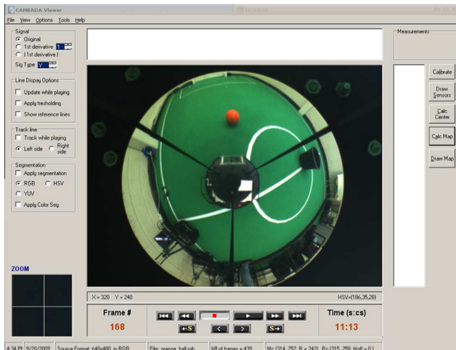
Fig. 7. A screenshot of the tool developed to calibrate some important parameters of the vision system, namely the inverse distance map, the mirror and robot center and the regions of the image to be processed.
