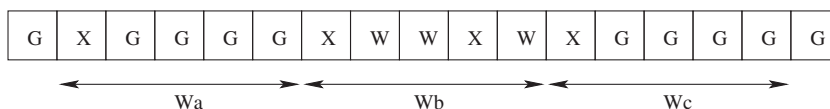
Fig. 14. An example of a transition. “G” means green pixel, “W” means white pixel and “X” means pixel with a color different from green or white, for example resulting due to some noise or a not perfect color calibration. (For interpretation of the references to color in this figure legend, the reader is referred to the web version of this article.)
