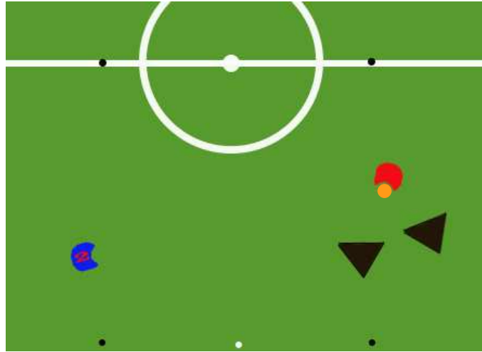
Figure 4.10: Conditions in which a pass should be made in free play. The red robot is the Striker, the blue robot is the Receiver and the black ones are the opponents.
