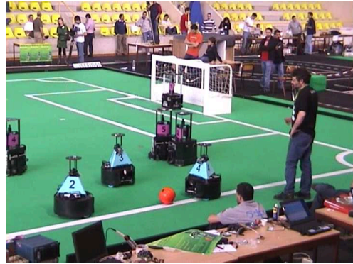
(b) Real game positioning - Robot 4 is the Replacer and robots 2 and 3 are the Receivers
