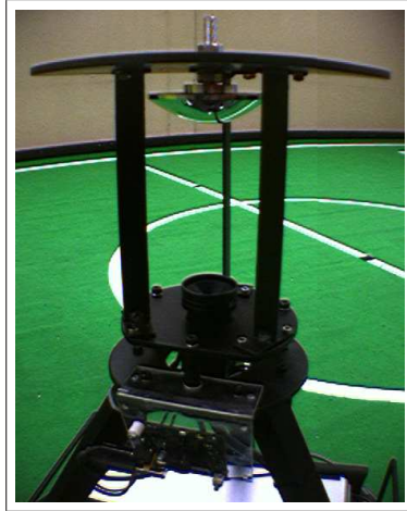
Figure 2.1: The hardware architecture of the vision system developed for the CAMBADA robotic soccer team. On the top, the omnidirectional sub-system with a camera pointing to an hyperbolic mirror. At the bottom of the image, the perspective sub-system with a camera pointing towards the field.
