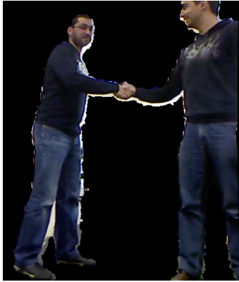
Fig. 5. The result of people extraction phase, fusing both the depth and color image of the Kinect. This is a debug image with all detected people. There will also be an image for every person detected.
