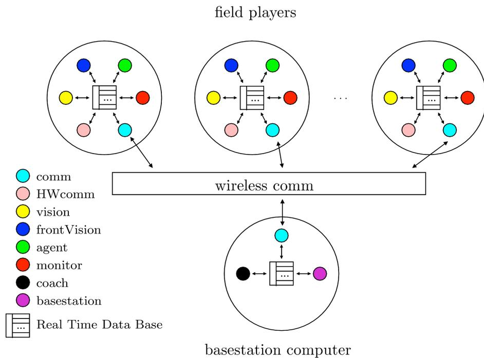
The Realtime Data Base (RtDB) is a middleware that provides a seamless access to the complete team state using a distributed database, partially replicated to all team members.
