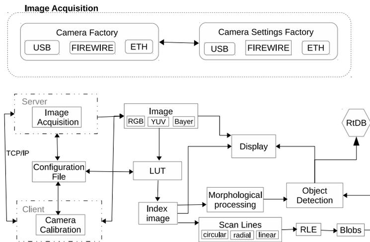
**Fig. 2.** Common vision library (UAVision) for UA robotic projects to be used in CAMBADA.
