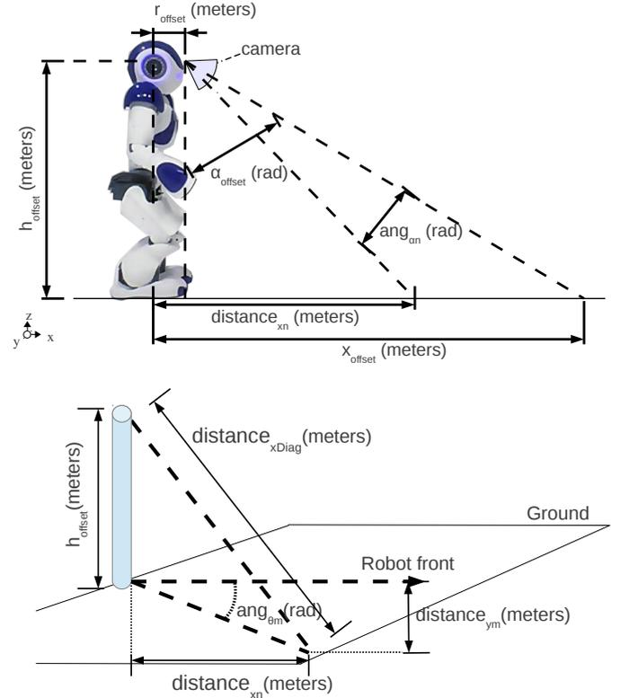
Figure 1: On top, side view schematic of the vision system. On bottom, a semi top view schematic of the vision system.
