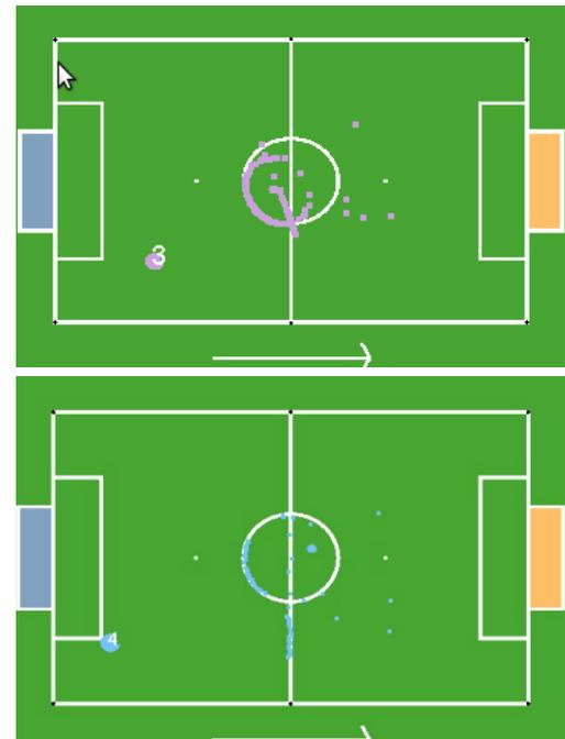
Figure 3: On top, the projection of points over the center circle using the projection without camera angle corrections. On bottom, the projection of a similar set of points now using the correction of the camera angles extracted through camera calibration tool.
