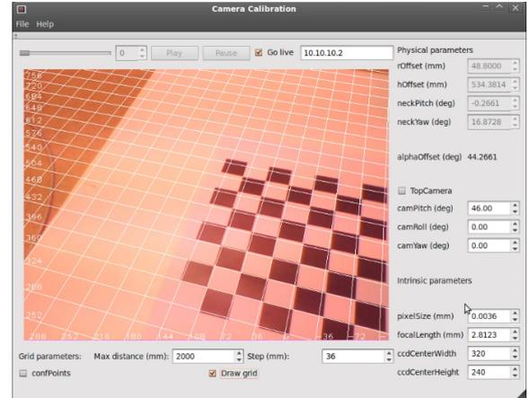
Figure 2: On top, the setup with known measures. On bottom, the 36mm grid projected on the image, with some pitch and yaw applied to the robot head.
