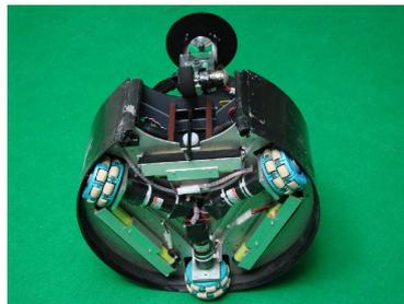
**Fig. 2.** Detail of the wheel configuration which enables an holonomic motion.
