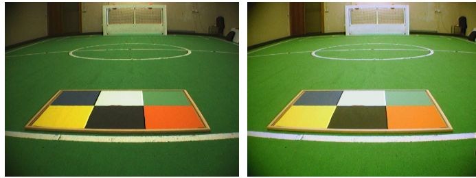
Figure 2.7: Examples of images acquired in the robotic soccer field with different values of gamma. On the left, an image acquired with a low value of gamma. On the right, an image acquired with a higher value of gamma.
