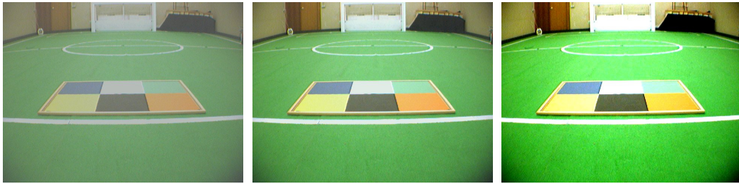
Figure 2.4: Examples of images acquired in the robotic soccer field with different values of contrast. On the left, an image acquired with a low contrast. In the center, an image correctly acquired. On the right, an image acquired with a high contrast.
