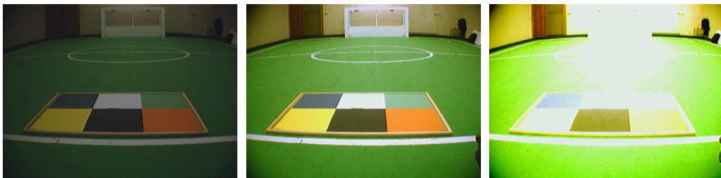
Figure 2.5: Examples of images acquired in the robotic soccer field with different values of gain. On the left, an image acquired with a low value of gain. In the center, an image correctly acquired. On the right, an image acquired with a high value of gain.
