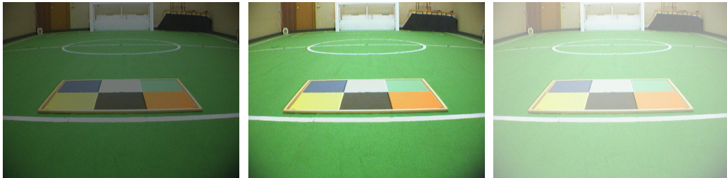
Figure 2.3: Examples of images acquired in the robotic soccer field with different values of brightness. On the left, an image acquired with a low value of brightness. In the center, an image correctly acquired. On the right, an image acquired with a high value of brightness.
