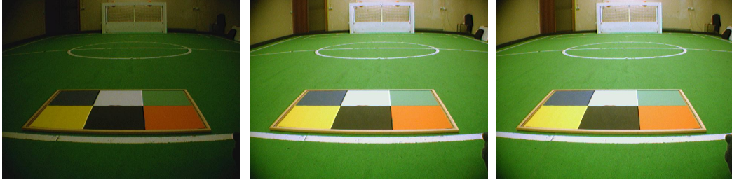
Figure 2.6: Examples of images acquired in the robotic soccer field with different values of exposure. On the left, an image acquired with a low value of exposure. In the center, an image correctly acquired. On the right, an image acquired with a high value of exposure.
