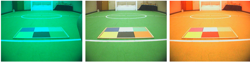
Figure 2.2: Examples of images acquired in a robotic soccer field using different values for the white-balance. On the left, an image acquired with a high value of the blue gain. In the center, an image with the white-balance correctly calibrated. On the right, an image acquired with a high value of the red gain.
