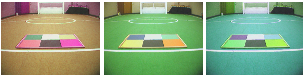
Figure 2.9: Examples of images acquired in the robotic soccer field with different values of hue. On the left, an image acquired with a low value of hue. In the center, an image correctly acquired. On the right, an image acquired with a high value of hue.
