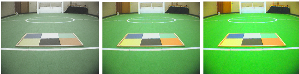
Figure 2.8: Examples of images acquired in the robotic soccer field with different values of saturation. On the left, an image acquired with a low value of saturation. In the center, an image correctly acquired. On the right, an image acquired with a high value of saturation.
