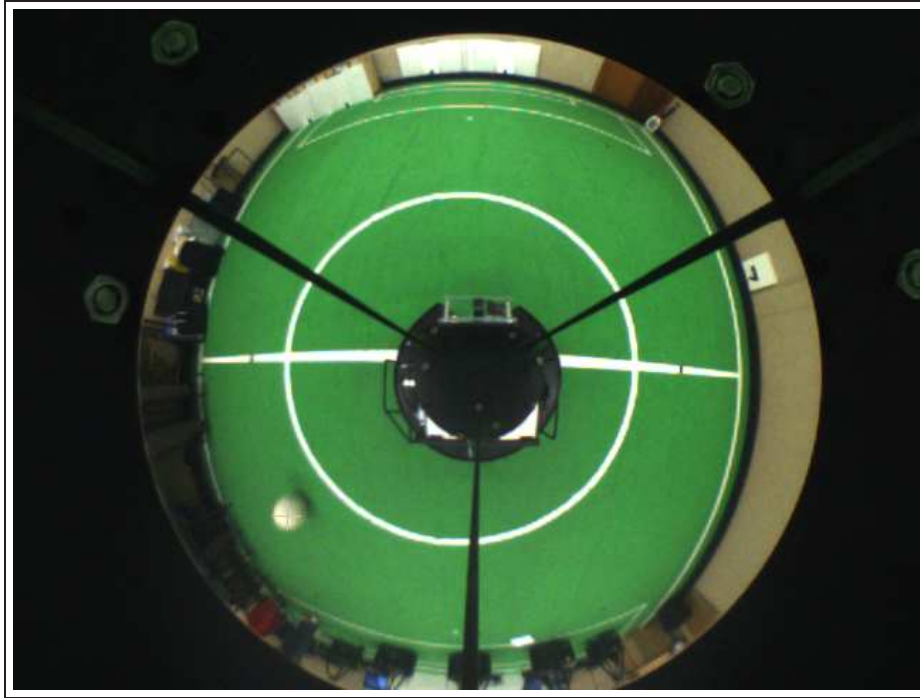
Figure 4.7: Example of a captured image using the morphological ball detection system. The cross over the ball points out the detected position.
